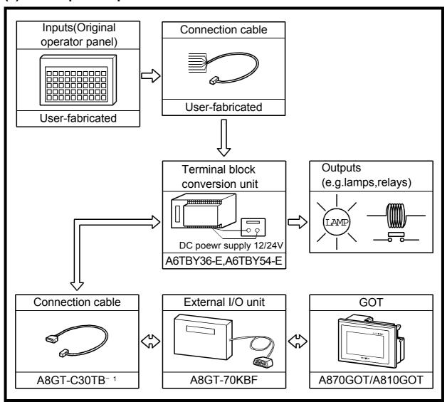
•1 The cable for connection between external I/O unit and terminal block conversion unit may also be fabricated by the user.
