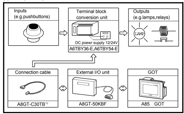
•1 The cable for connection between external I/O unit and terminal block conversion unit may also be fabricated by the user.
